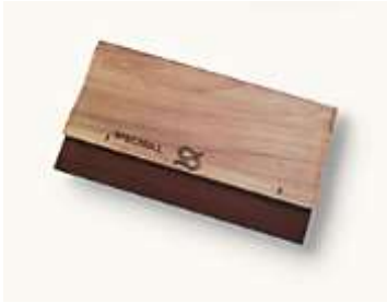
Squeegee: Used to push the ink through the openings in the screen
