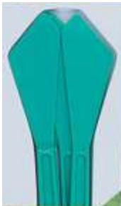
Palette Knife: Used to get ink out of the jar and to push small hits of color through the screen.
